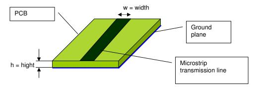
If the antenna connector is mounted on the chassis, a 50 Ohm coaxial cable must be used from the module to the connector. A metal chassis is preferred as this will act as a ground plane. The coaxial cable shield should be connected to the chassis. If the chassis is non-conducting, a conducting (metal) plate should be placed at the base of the antenna to act as the ground plane.
